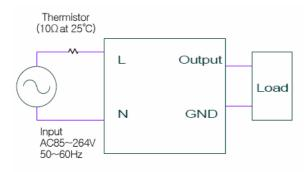
NOTE: To avoid excessive voltage drop and for Improved noise, short and thick wire should be used to connect the load. Length below 50Cm & wire thickness of 4.0A/mm² are recommended for reducing wire loss when wire connection is necessary.
